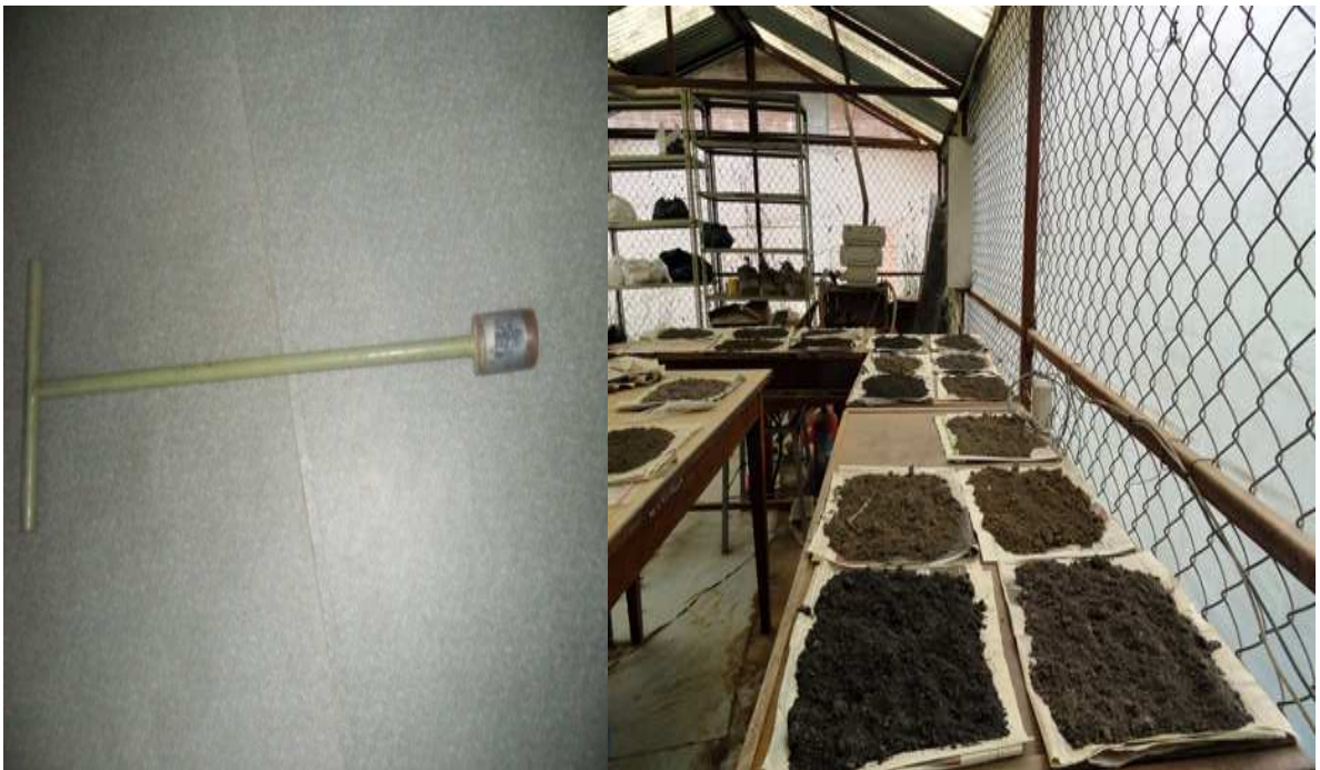
Picture 5 I. Soil core sampler II. Drying of soil samples in shed
