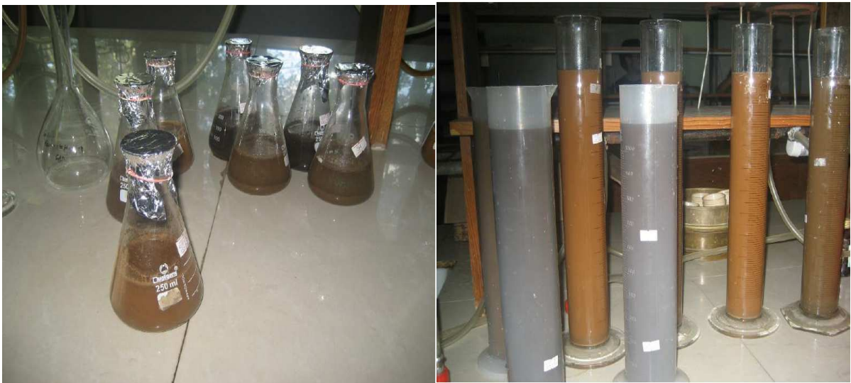
Picture 7 Soil texture determination steps, (I), soil sample soil mixed with sodium hexa-metaphosphate and water (II), texture determination
